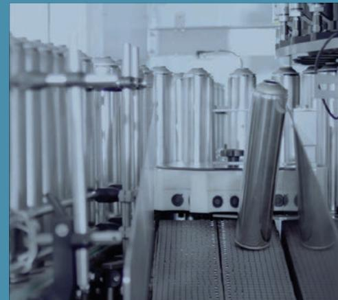
Aluminium was introduced in the 1960s with single-piece cans, a cylinder obtained by tapering an aluminium tablet. The upper edge is curled where the filled cylinder valve is crimped.
